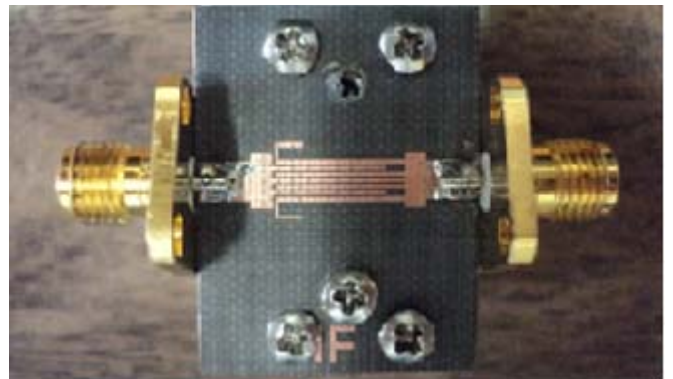
Figure 8. Fabricated dual band-notched (2 nd and 3 rd harmonics of 2.14 GHz) UWB bandpass filter.
